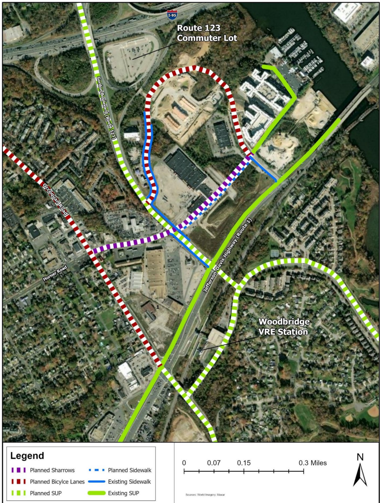
Figure 3-6: Existing and Proposed Pedestrian Facilities
