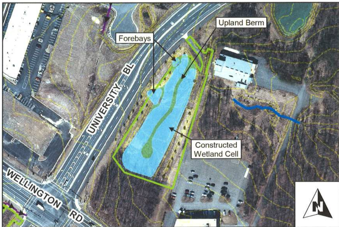
Conceptual Plan: Conversion to a wetland will increase N and P removal. Facility includes forebays for pretreatment and a berm to increase flow path.
