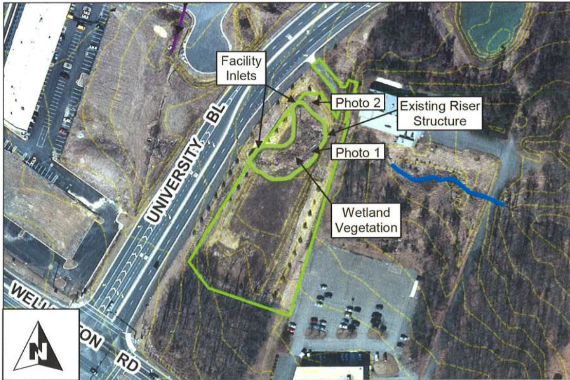
Existing Condition: Facility designed as a dry pond is supporting wetland vegetation due to clogged low flow orifice. Flow has a short path to outlet structure.
