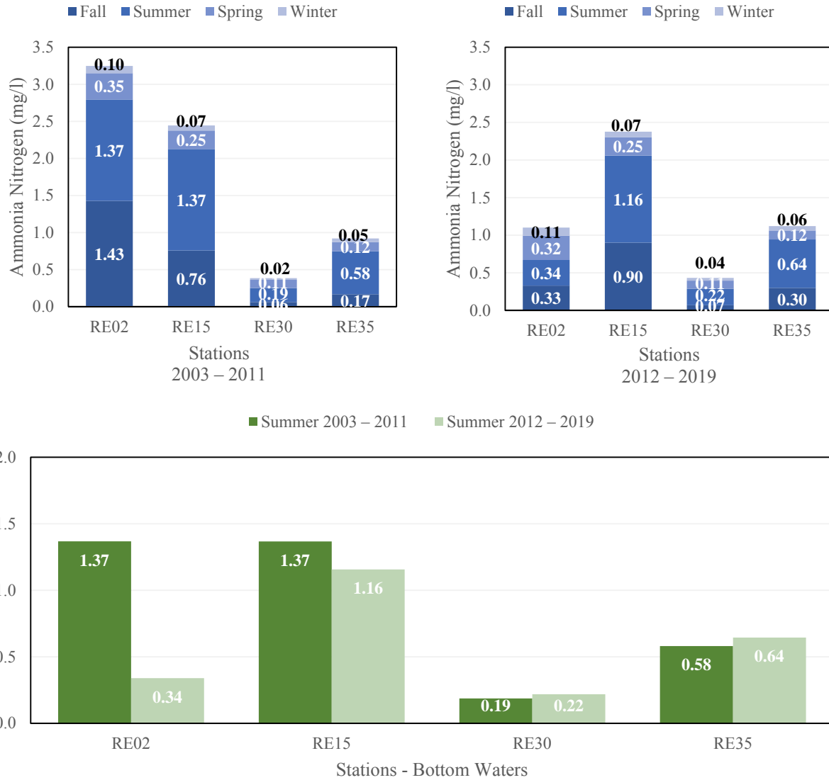
Figure 4-67. Seasonal Average Ammonia - Before and After Installation of Hypolimnetic Oxygenation System
